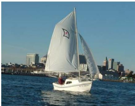
*For running downwind, poling out the jib on the opposite side so as to uncover the jib from the windshadow of the mainsail is a standard technique.*
