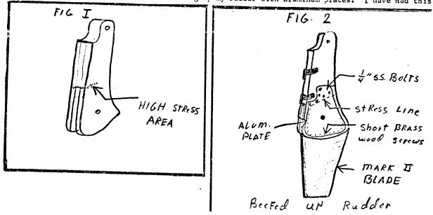
for three years now, and it is still 'bullet-proof'. I used 1/8" thick aluminum plates, 6061 grade; 7½" stainless steel bolts, and about 25 small brass wood screws. See Fig. 2. I have a template made (cardboard) for Mark I rudders. If you can't find any material, give me a call (828-3572).
